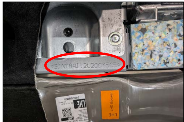
VIN stamped under the Front Right Seat on the frame underneath the cover
